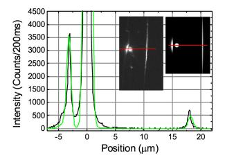
FIG. 3. Intensity of PL emitted from the film under spot excitation as recorded by the EM-CCD camera. (Left inset) Experiment. The bright circle is due to emission from the directly excited region of the film. (Right inset) Simulation. (Main figure) Profile of PL intensity across the film at the location indicated by the red line in the insets. The black (green) line is the experimental (simulation) result. Spot excitation is at  $0 \, \mu m$ .
