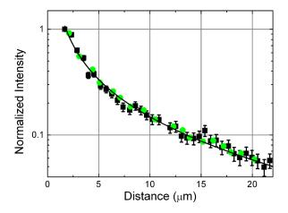
FIG. 4. PL intensity from the crazed region as a function of distance between the excitation spot and craze. Experimental (simulation) results are indicated by black squares (green circles). The black line is the result of fitting the experimental results to an exponential-circular decay curve with  $r_o = 40\mu m$ . Simulation was conducted using the measured absorption and PL spectra and a scattering length ( $l_s$ ) of 100  $\mu m$ .
